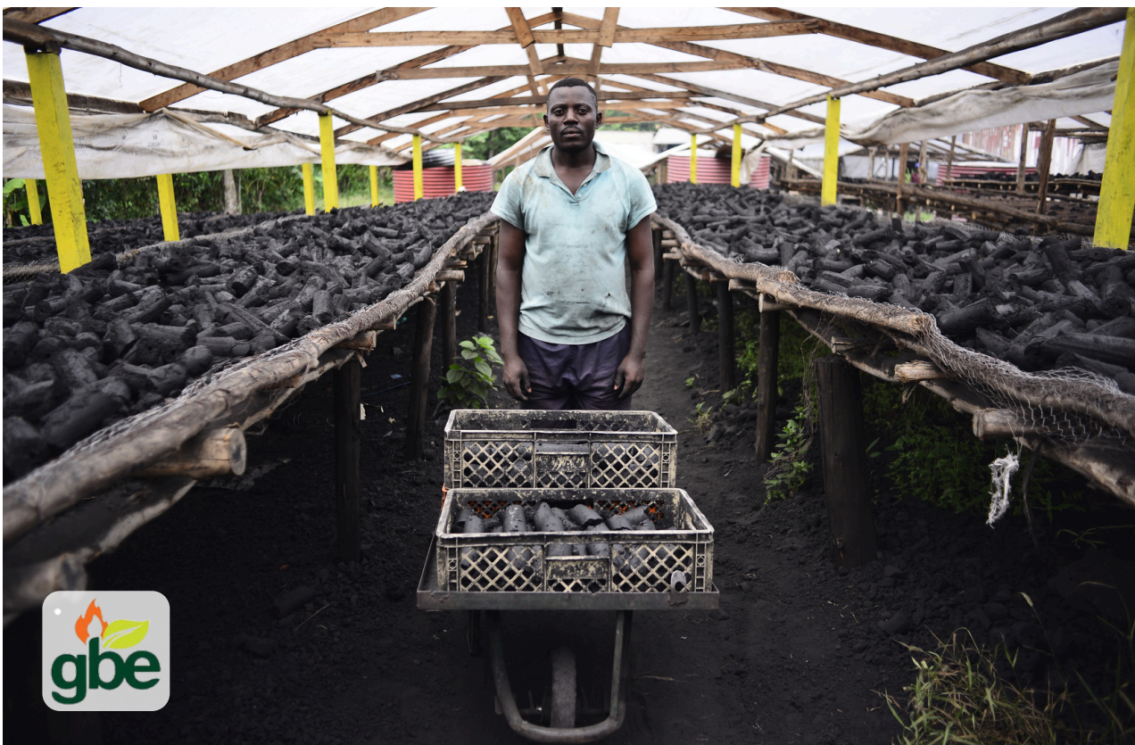
Briquettes laid out on solar dryers at GBE's briquettes facility in Mukono, Uganda Photo Credit: Charles Sabourin
